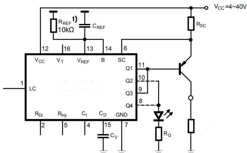
Remark: External PNP structure output with short circuit protection and LED indication. Generally, the short circuit protection is calculated by using the following equation:
