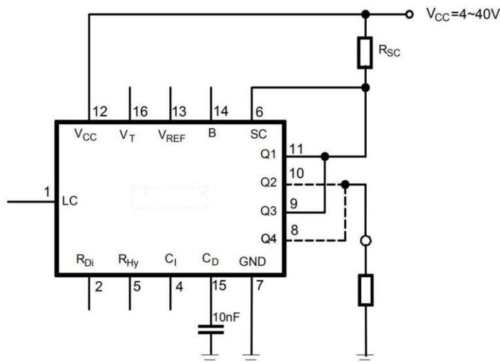
Note: Direct internal NPN output structure with short circuit protection and LED indication. Generally, the short circuit protection is calculated by using the following equation:
