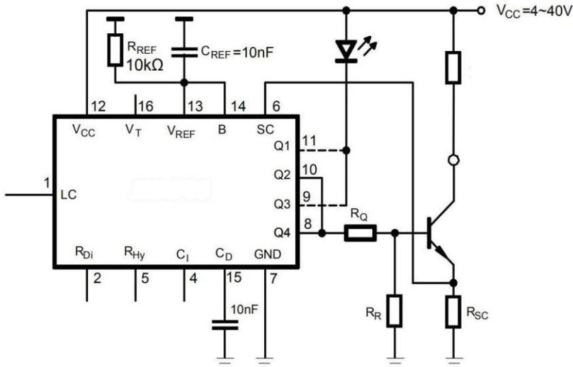
Remark: External NPN structure output with short circuit protection and LED indication. Generally, the short circuit protection is calculated by using the following equation:
