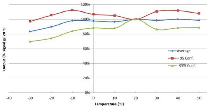
Figure 5.1. Sensor Sensitivity Temperature Dependence
