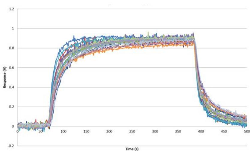
Figure 4.2. Sensor response to 50ppm NH3
