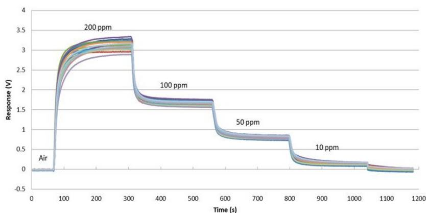
Figure 4.1. Sensor response to NH3 Gas with Various Concentrations
